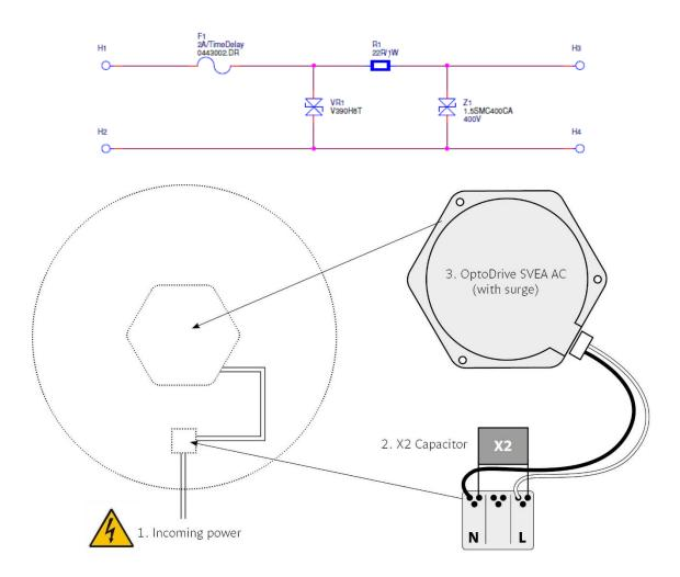
The installation set up requires an X2 Capacitor parallel to L1 and N to handle the fast and high voltage transients generated by the magnetic ballast.
