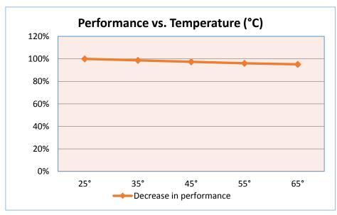
Consider the thermal capabilities of where the LED module is to be fitted. The temperature is an important factor for light output as well as for long time light output degradation.
